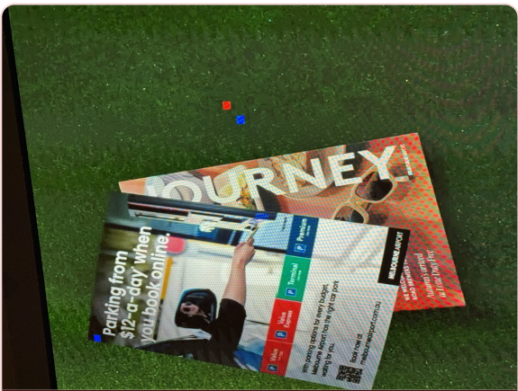
FIG 8 Stuck pixels (1× red, 2× blue) caused by data-connection solder faults on the receiving card — the data signal to those pixels has been lost while power remains intact.
