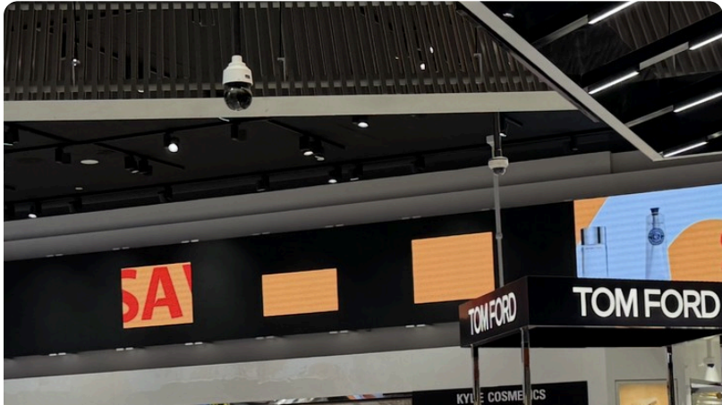
FIG 6 Dropped cabinets in a live ribbon — chassis-to-chassis connector and data-interconnect failure: the data hand-off between cabinets has been lost at the connector while power to the affected cabinets remains intact.
