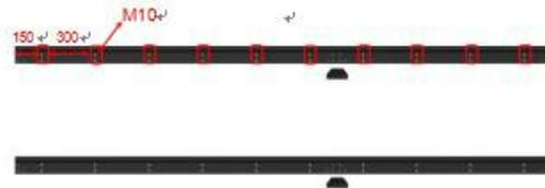
4) Mark the corresponding hole positions. Punch at the marked points with a tool. Each hole is sized 10 mm in diameter;
