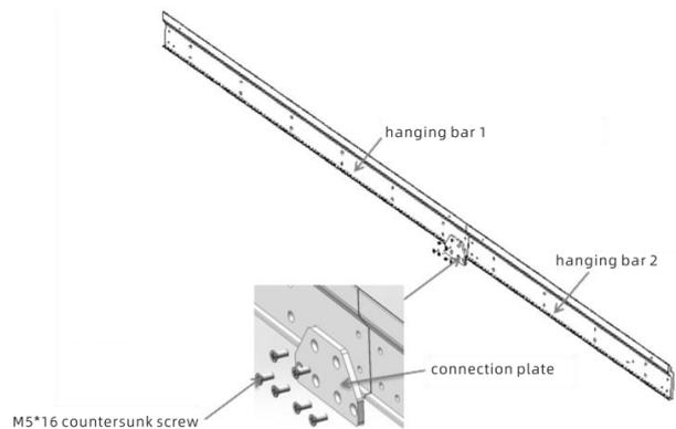
2) Install the hanging bars on the bracket, as illustrated below:
