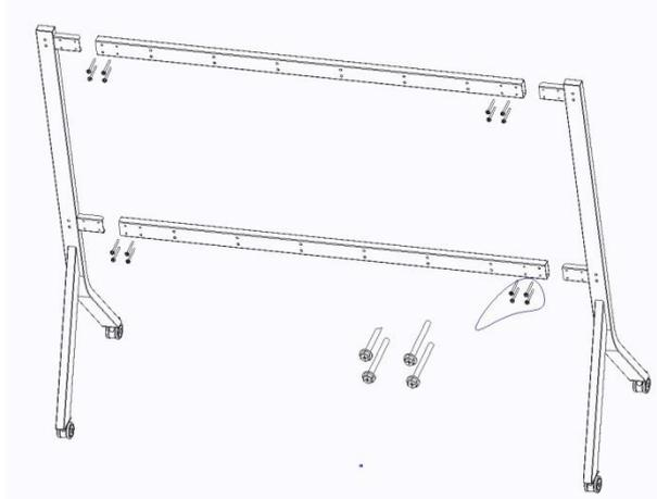
2) Tighten the installation screws with the corresponding tools. The assembled bracket is as shown below:
