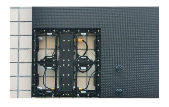
3. After removing all 4 modules from one cabinet unplug the signal and power cables.
