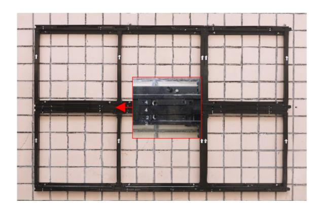
7. Move the positioning slider on the adjustment frame to ensure wall mounts are even with the ajoining wall mounts.
