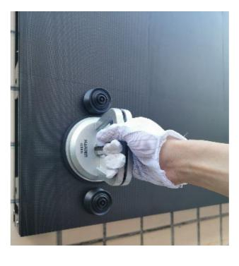
2. Remove module using the maintenance tools
